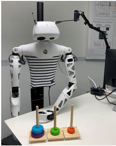
Fig. 1. Experimental setup from the child's viewpoint, showing Reachy behind the Tower of Hanoi puzzle, mid-solution. The child sits across from Reachy where they can both reach the game to play collaboratively. Sessions were recorded using the webcam mounted to the right of Reachy's head in the image. The researcher was seated behind the monitor with their face and upper body blocked from the child's direct view.
